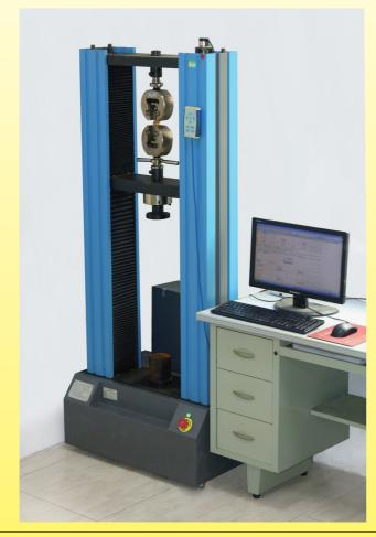
Tensile strength and elongation at break equipment
