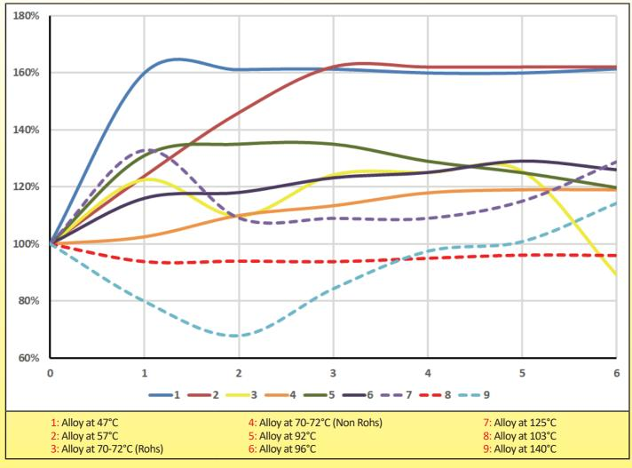
The above curve represents the variation of the resistance, in % of the value measured immediately after soldering, over 6 weeks, of welded test specimens, using a 225mm² surface weld, made with various fusible alloys.
