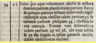
1701 description of an alloy comprising 2 parts of lead, 3 parts of tin and 5 parts of bismuth by Isaac Newton in "Scalum graduum caloris"
