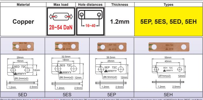
These fusible links have a medium response time, between 3 minutes 25 seconds and 3 minutes 30 seconds, for a temperature rise rate of 20°C/min from 25°C, and their thickness of metal is thicker than brass models to gives them sufficient strength for their use in multiplied mechanisms supporting a maximum stress of 300DaN. The use of red copper instead of brass provides a better corrosion resistance but substantially increases the price.
