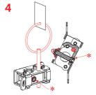
4/ Tighten the screw with a torque controlled wrench.
