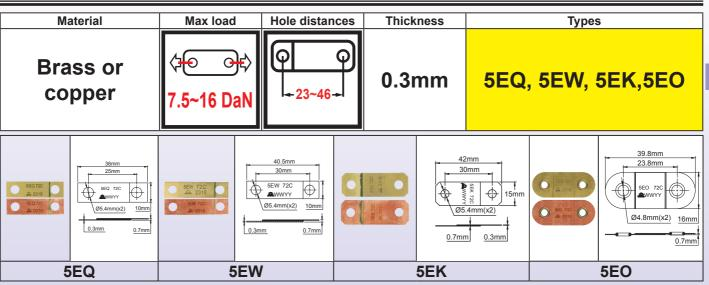
Made of thin metal, these fusible links have the shortest response time, between 2 minutes 50 seconds and 3 minutes, for a temperature rise rate of 20°C/min from 25°C, but the fineness of the metal limits their mechanical strength.
