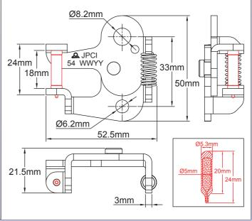
Made of 3mm thick galvanized steel, these reduction mechanisms are compatible with 20x5mm thermal glass bulbs. Their huge multiplying coefficient reduces the force applied to the thermal glass bulb to only 15% of that applied to the mechanism. The replacement of the glass bulb is simple and can be done without special tools.
