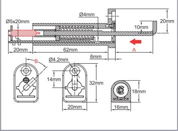
These mechanical thermal actuators are intended to close the fire dampers used on the ventilation ducts. Their large operating force unlocks the spring actuating the damper. Requiring no power supply, these devices are particularly simple and reliable. They are mandatory for all fire dampers to meet the NF-S 61.937 standard. Since thermal bulbs are not subject to creep, their periodic replacement is not necessary.
