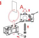
3/ Put carefully a new glass bulb inside (Dia.5mm). Put the screw and tighten lightly it by hand. Don't break the bulb filling needle. If any doubt, unclip the bulb needle cap (A) with a small screw driver, and check visually that the filling needle is not broken. Do not miss to clips again the cap after inspection.
