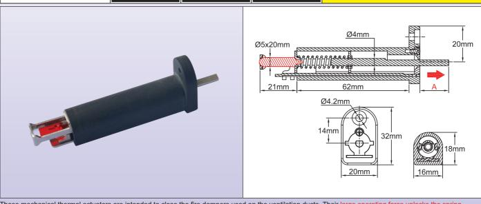
These mechanical thermal actuators are intended to close the fire dampers used on the ventilation ducts. Their large operating force unlocks the spring actuating the damper. Requiring no power supply, these devices are particularly simple and reliable.
