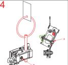
4/ Tighten the screw with a torque controlled wrench.
