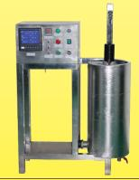
Automatic control equipment for checking the minimum force of thermal links in our laboratory
