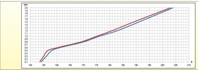
Average threshold response time and threshold temperature on the full range of existing models against thickness, soldered with non-Rohs eutectic alloy at 72°C
