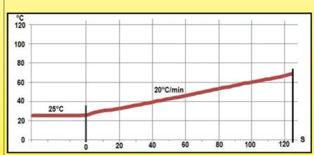
Position of the thermal links or thermal bulbs mechanisms in the air stream for threshold temperature limit measurement Example chart of temperature rise at 20°C per minute, starting from a plateau at 25°C
