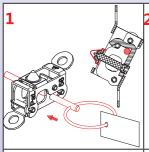
Glass bulb replacement must be made by trained technicians. Only genuine glass bulbs with the same calibration temperature must be used.
