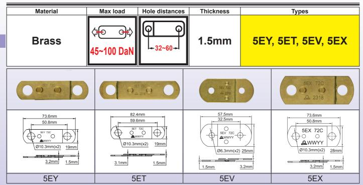
These fusible links have a response time near the highest limit requested by standard (whose threshold is 4 minutes), between 3 minutes 30 seconds and 3 minutes 50 seconds, for a temperature rise rate of 20°C/min from 25°C. Their 1.5mm metal thickness and their soldering surface make it possible to withstand directly and without multiplying mechanism the loads encountered in the opening or closing mechanisms of fire doors and shutters.
