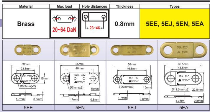
These fusible links have a medium response time, between 3 minutes and 3 minutes 10 seconds, for a temperature rise rate of 20°C/min from 25°C and their thickness of metal gives them sufficient strength for their use in multiplied mechanisms supporting a maximum load of 300DaN. The holes have a lip to improve their resistance to mechanical break at 25°C by avoiding the tearing of the metal.
