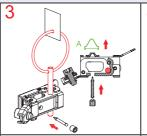
3/ Put carefully a new glass bulb inside (Dia.5mm). Put the screw and tighten lightly it by hand. Don't break the bulb filling needle. If any doubt, unclip the bulb needle cap (A) with a small screw driver, and check visually that the filling needle is not broken. Do not miss to clips again the cap after inspection.
