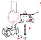
2/ Remove the screw with hexagonal key wrench. Size is 2.5mm for 58L, and 1/8 inch, (3.17mm) for 58Z. Remove the old glass bulb.
